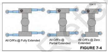
The shortest outrigger position determines the chart that is to be used. For example:
