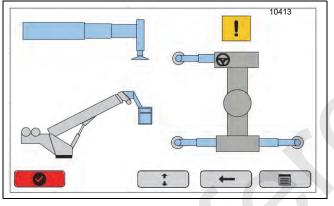
If the user selects a setup configuration different than the predefined selection given by the RCL, the O/R override icon is displayed on the confirmation screen and on the RCL Operating Mode Screen shown on page 7-10.
