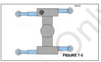
If any of the Outrigger Length Monitoring Sensors are out of range or not functioning properly, that beam will be missing and an icon with an exclamation point will be shown.
