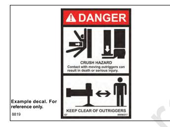
**Do not remove** the *Load Chart*, this *Operator Manual*, or any decal from this equipment.
