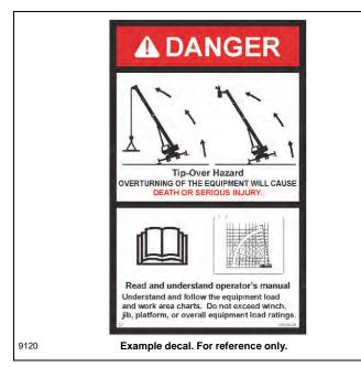
Carefully follow the procedures in this Operator Manual when extending or retracting the outriggers. Death or serious injury could result from improper equipment setup on outriggers.
