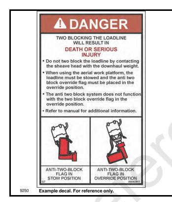
Two-blocking is more likely to occur when both the main and auxiliary hoist lines are reeved over the main boom nose and jib nose, respectively. An operator, concentrating on the specific line being used, may telescope or lower the boom allowing the other hoist line attachment to contact the boom or jib nose, thus causing damage to the sheaves, or causing the hoist rope to fail, dropping the lifting device to the ground and possibly injuring personnel working below.
