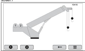
Select 1 to show the Main Hoist enabled. Select 2 to show the auxiliary hoist enabled.
