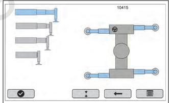
Select the check mark after machine is in outrigger setup configuration without jib or personnel platform with 75% extended.
