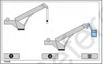
Is a personnel platform attached to the boom or the tip of the jib nose? Select 1 (no) or 2 (yes).
