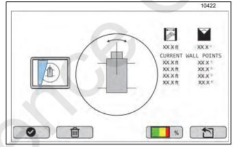
There can be up to four set points which form 3 virtual walls. The points are taken from the slew angle and calculated radius.
