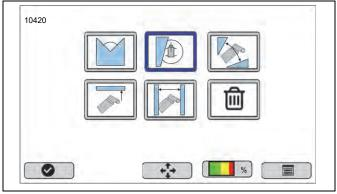
Select the desired operational limit 1 through 6. Use the arrow key to scroll back and forth to select the correct operational limit.
