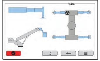
If the user attempts to select the check mark before the Fully Extended condition is met, the check mark button is missing. The user can override the setup using the arrow keys and the check mark.
