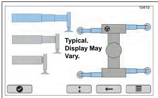
The current outrigger status is displayed by highlighting the current outrigger setting in blue, as shown in the left view of Screen 6. The non-current span setting is shown in gray.
