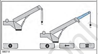
Is a jib attached to the boom nose? Select 1 or 2.
