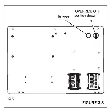
The RCL is bypassed only as long as the switches are in the ON position. When overridden, warning icons appear on the RCL display. For more information, see "About the RCL and ATB Override Warnings" on page 7-6.
