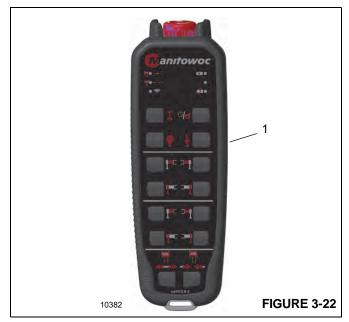
The rigging Remote Control (1, Figure 3-22) is a palm size remote control and is shipped with each crane as optional equipment. This rigging remote control has limited functions as described in the following sections; it does not allow full remote control of the crane.
