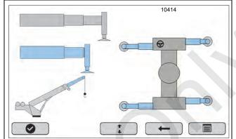
If the user attempts to select the check mark before Fully Extended, 75%, or 50% Extended condition is met, the check mark button is colored RED when depressed and the user can override the setup using the arrow keys.
