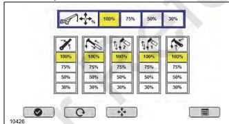
• The operator can also set the desired output for each function as shown in Controller Output #3 screen.
