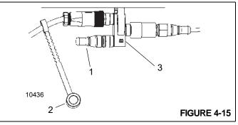
**4.** Remove the resistor (1, Figure 4-15) from the cap (2). Install the resistor in splitter port B (3).
